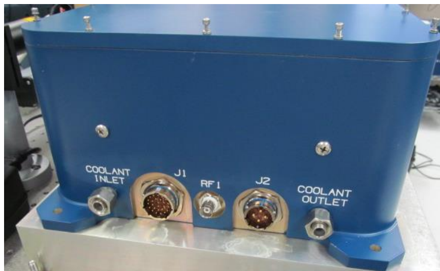
Figure 4-5 Connectors on the rear panel of the Iklwa laser (Gen II)
