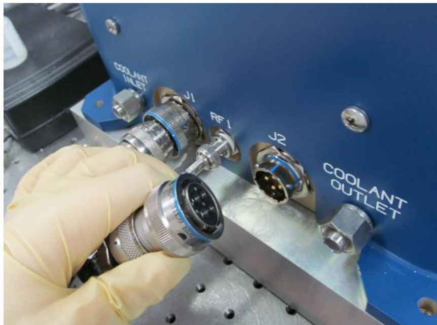
Figure 4-11. Diode Power Connection (Gen II)
