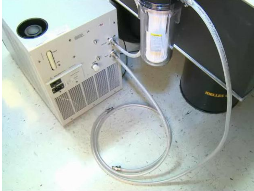
Figure 4-3. Chiller Assembled with Water Hoses and Filter
