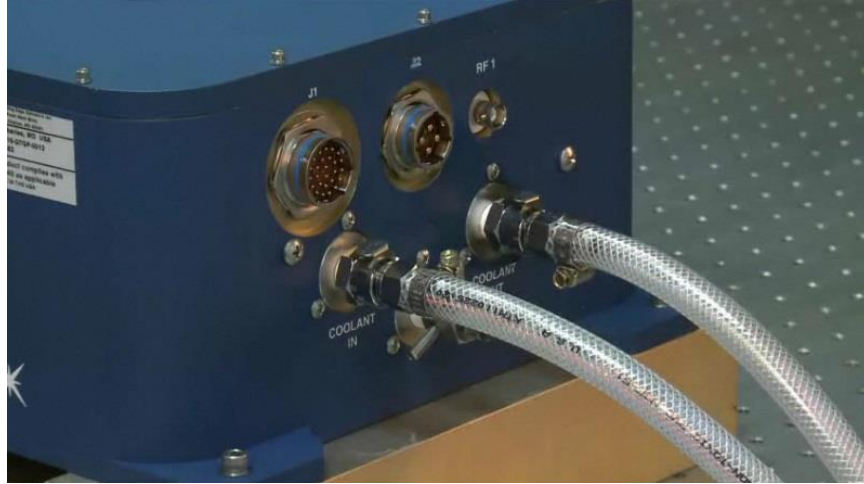
Figure 4-6. Plumbing Connection (Gen I)
