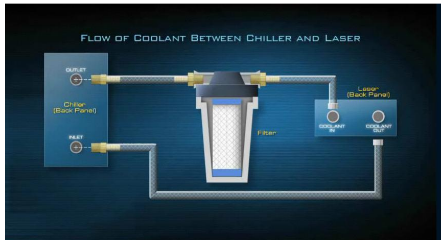
Figure 4-2. Water Hoses and Filter Connections
