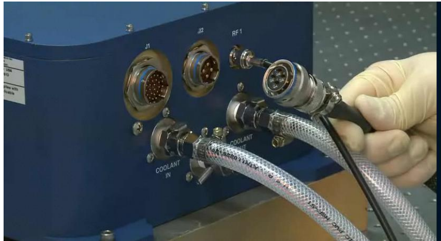
Figure 4-10. Diode Power Connection (Gen I)
