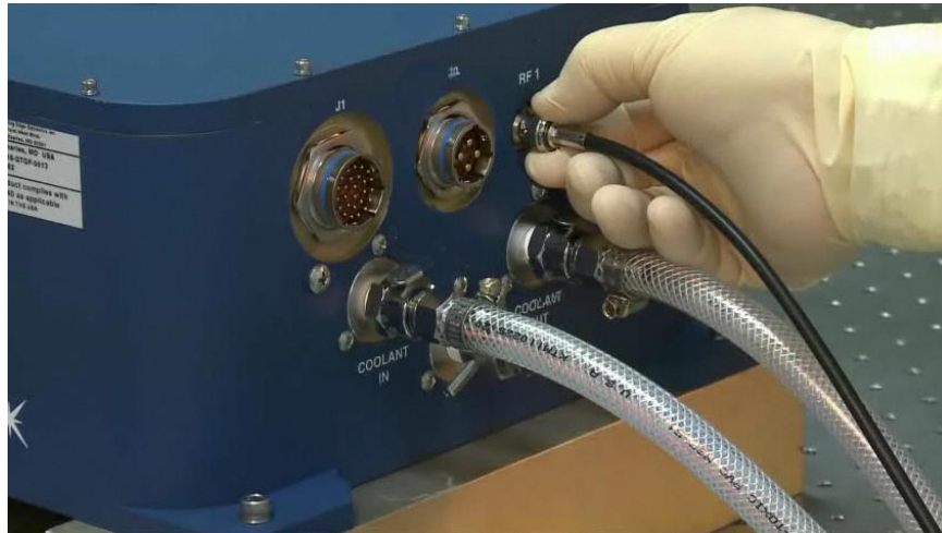
Figure 4-8. RF Connection (Gen I)
